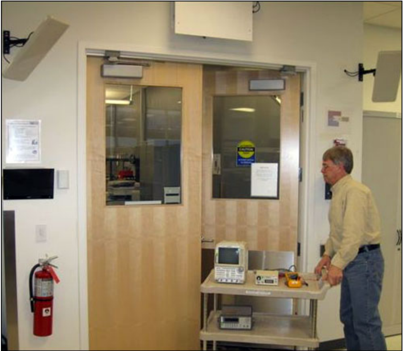
Dave Erenberg, the ESD division's principle design technician, pushes a cart loaded with tagged equipment through a lab's RFID portal.
