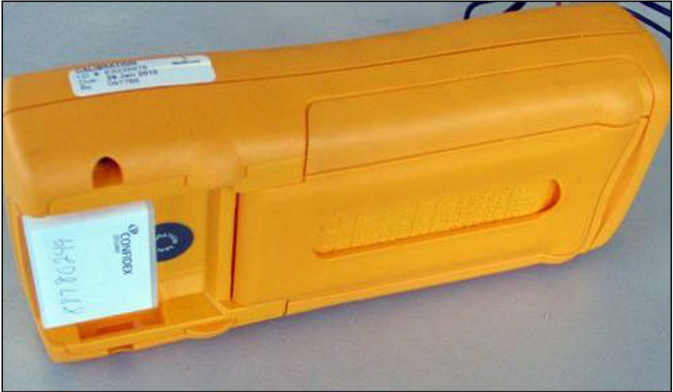
A meter fitted with a Confidex EPC Gen 2 passive RFID tag
